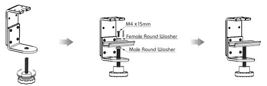
Assemble C Clamp with Mount by driving 4 Screws M5x14mm, flap head, Hex Socket Screws.
